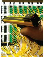
Another common application for the PX-Q500 is end to end fiber tracing. Working in tandem with a 2kHz tracer source, the Flashpistol® probe can trace fiber links with overall losses in excess of 70, 80, or even 90dB. This level of performance represents an ability to trace even un-amplified fiber spans well over 350km in length.
