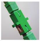
Similar to mated connector contamination or damage detection, the PX-Q500 will detect leakage radiating from around a bulkhead adapter if it has a damaged or contaminated alignment sleeve or if the connectors inside are not fully engaged with one another. IR radiation can be detected through many plastic bulkhead adapters or from the leeward boot areas of a mated connector pair.
