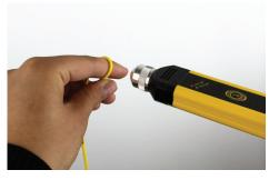
Bending a patch cord or buffered fiber over a wide mandrel or finger will extract enough tracer light from a fiber to permit detection with the PX-Q500. Such a minor bend, while enough to trace with, will induce far less attenuation in a fiber than the clamping heads on most fiber identifiers. This gentle bend is easier to perform in the field and is less likely to cause signal drop out on active fibers.
