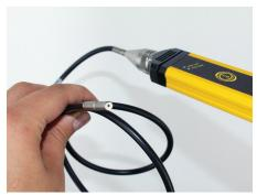
In the field, rodent damage under telephone pole riser guards or conduit entrances can sometimes be detected using the optional PX-Q731 24" flexible adapter head. By pushing the tip of the flexible fiber bundle into the tube, it is possible to detect stray radiation scattered from rodent chew points.
