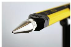
Vintage ribbon fibers sometimes have a problem with color code fading. This presents problems with restoration or splice repair when it comes to determining ribbon orientation. By placing a tracer signal on "fiber 1" at the CO or head end, the PX-Q500, fitted with a PX-Q721 fine point tip can be used to locate which strand is actually "fiber 1" in the field ribbon.
