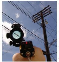
Aerial damage due to firearms, rodents, birds, or arcing can be detected using the PX-Q550 Flashpistol<sup>®</sup> or the PX-Q650 Flashfinder<sup>™</sup> aerial leak detection probes. The PX-Q550 is specialized version of the PX-Q500 which has been optimized for long range leakage detection. The key additions which make the PX-Q550 unique are a 1550nm specific long range lens head for remote light collection and a red-dot sighting scope for proper aim.
