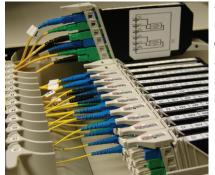
Splitters can be checked for damage by scanning in a method similar to that used for fiber bend and break testing. In addition, ports can be checked end on for the presence of light or by bending output fibers over a finger or mandrel. Splitters with division ratios as high as 1:32 are verifiable in this way due to the high sensitivity of the PX-Q550. WDM devices can also be tested with the use of narrow band heads to verify proper wavelength diversion.
