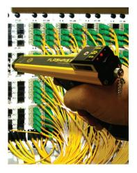
In situations where patch cords are connected to the output ports, simply bending patch cords over a finger will permit tracing. When used with Photonix high power tracer sources, the PX-Q550 can even trace ports through most plastic end caps or by connector bulkhead leakage.
