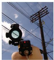
Aerial damage due to firearms, rodents, birds, or arcing can be detected using the PX-Q550 Flashpistol® or the PX-Q650 Flashfinder® aerial leak detection probes. The PX-Q550 is specialized version of the PX-Q500 which has been optimized for long range leakage detection. The key additions which make the PX-Q550 unique are a 1550nm specific long range lens head for remote light collection and a red-dot sighting scope for proper aim.
