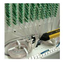
the PX-Q650 can also directly detect light leakage from broken splices, bulkhead adapters, broken or disengaged connectors, and fan-outs, even in bright ambient light conditions.
