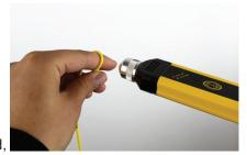
To test, attach a tracer source to the port of interest and simply bend the cord or cords under test over a finger to search for light leakage. Scanning over the bend,
